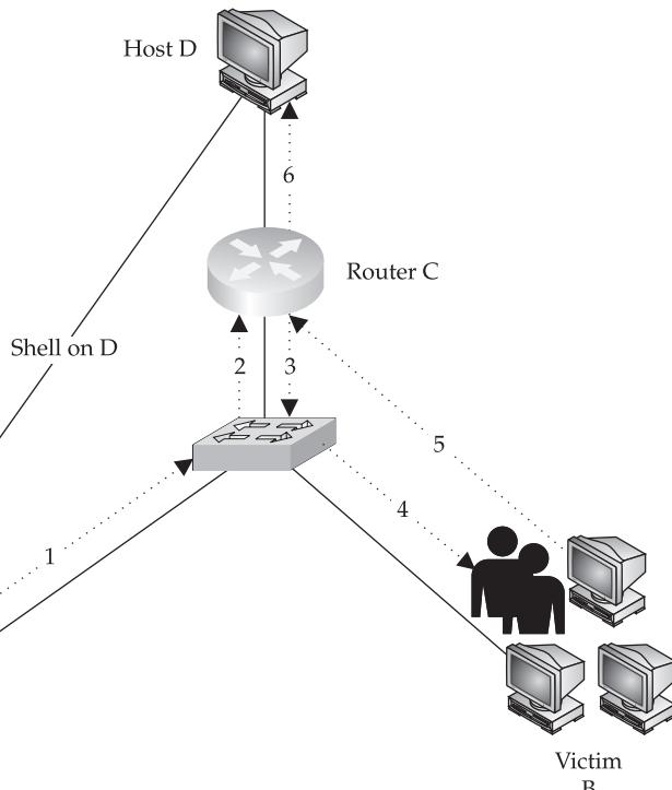
**Figure 12-9** Making use of a PVLAN hopping attack
